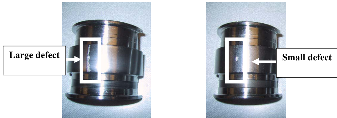
Figure 8 Seeded 'small' and 'large' defects on the inner race
